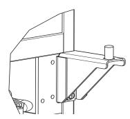
2. Remove corresponding screws on opposite side of cabinet. On some models there may be a nut behind one or both screws on either side.
